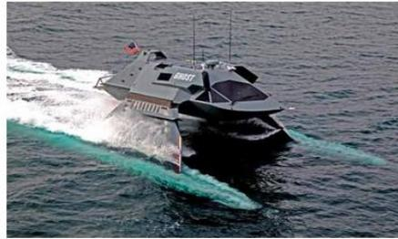
In defence technology, we will see more of drones and smaller crafts, very fast but with much lower G-forces (acceleration) as traditional boats. Their shape will be based on either wave-piercing hulls or SWATH (Small Water Area Twin Hull) or cross between both. And, they will be stealth.
